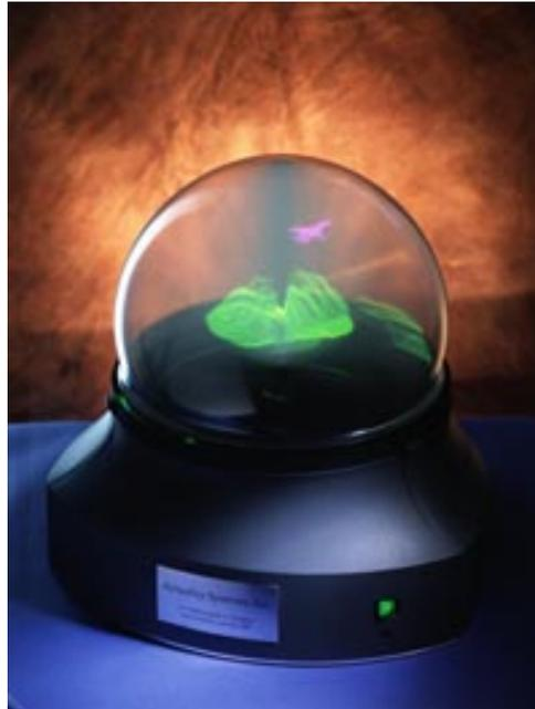
Figure 2. Perspecta volumetric display
