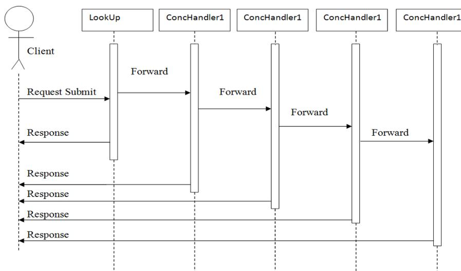
Figure 1. The sequence diagram of the “Obligation Link” design pattern
