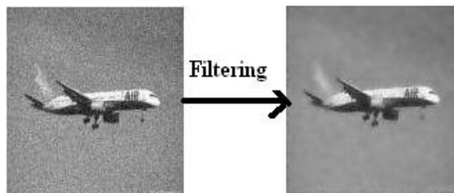
Figure 3. Applying Wiener Filter on noisy image
