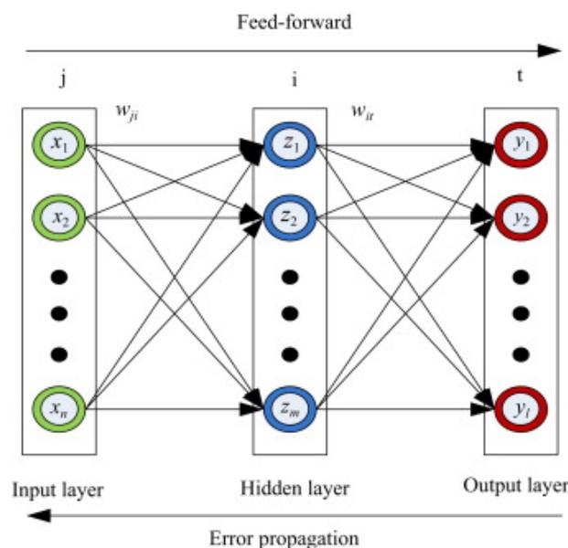
Figure 4. Feed Forward Back propagation Neural Network
