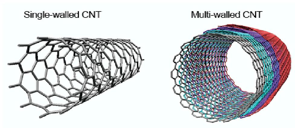
Figure 1: The structure of CNT
