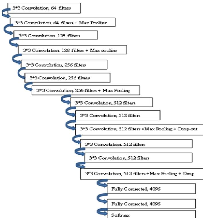
Figure 6. Basic DNN Structure.
