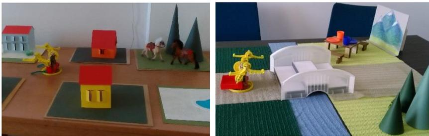
**Figure 7.** Initial set up (left) - the child controls the BigFoot robot via laptop interface, but pays attention to the toys outside eyesight; Walking robot BigFoot modified after Experiment 1 (right) – The robot is augmented with a platform to place the toys. The child controls its movements toward the toys via a joystick, so that the robot, the toys and the control are within the eyesight of the child
